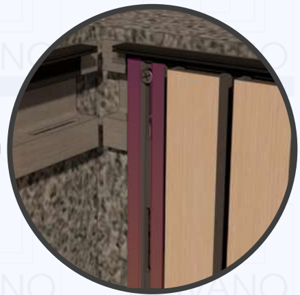
3 Apply PL Premium adhesive on this area to hold the cut female board.
